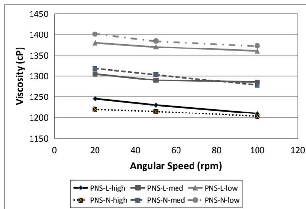
Figure 3. Viscosity measurements of the RPC produced with the six PNS-based superplasticizers at a 0.20 w/cm
