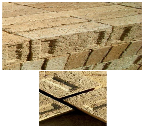
Figure 2. Brick made from Hempcrete [16]
