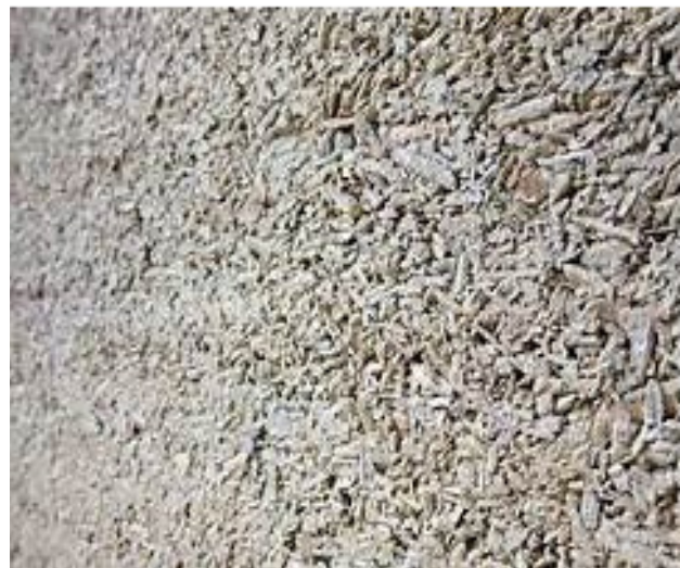
Figure 6. Hemp Concrete as insulating material
