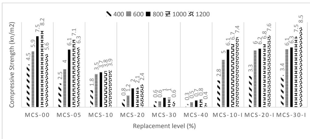
Figure 6. Compressive Strength (kN-m<sup>2</sup>)
