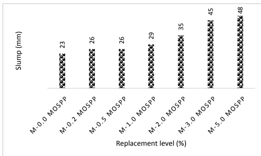
Figure 8. Slump of MOSP-Concrete
