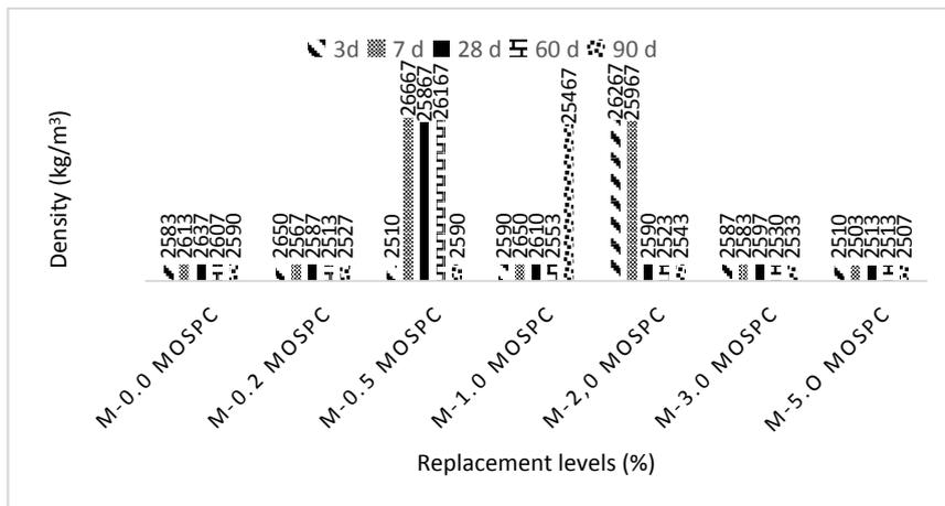
Figure 12. Density of MOSP-Concrete
