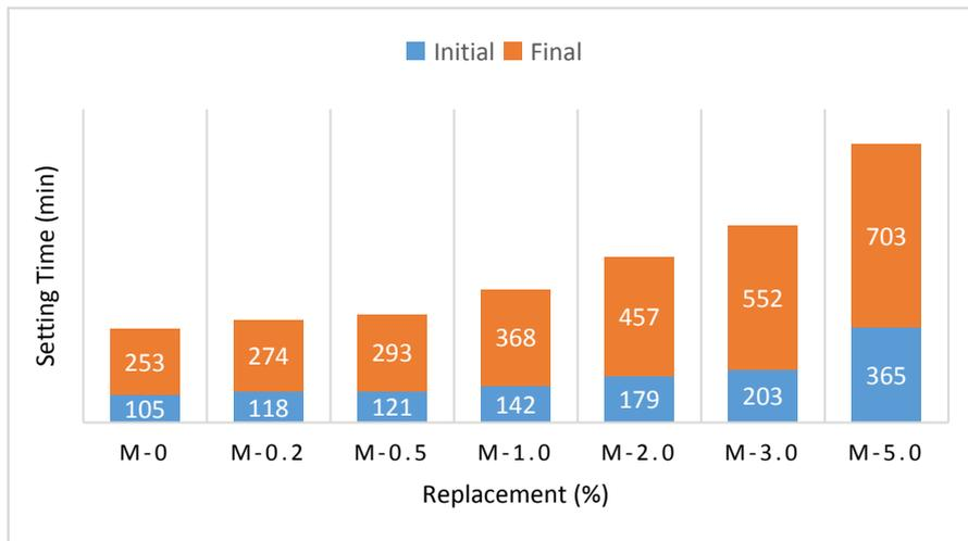
Figure 7. Setting Times of MOSP Cement Paste
