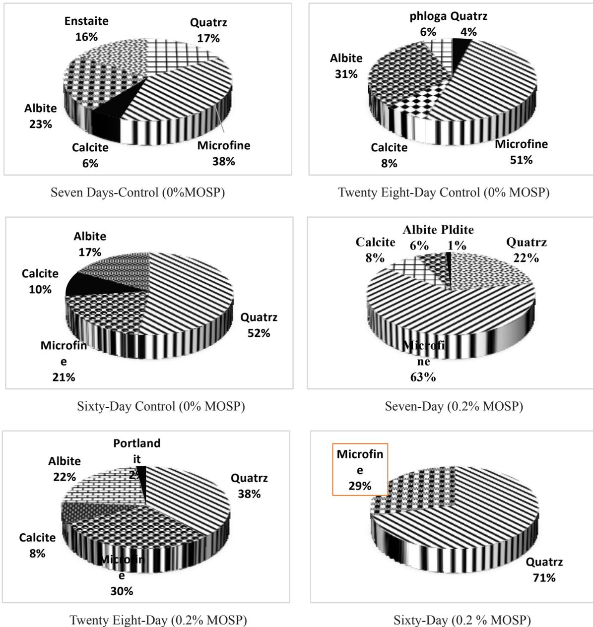
Figure 15. Characteristics of x-ray diffraction peaks of MOSP-concrete
