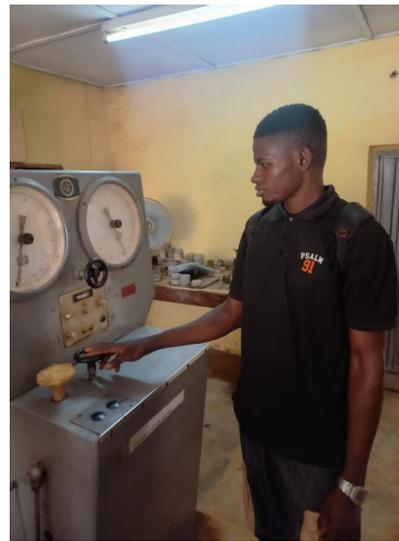
Plate 4. Compressive Testing Machine during Crushing
