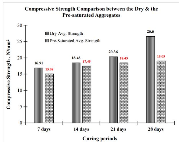
Figure 8. A Clustered Bar Chart Showing the Comparison between the Compressive Strengths of Dry and Pre-Saturated Coarse Aggregate
