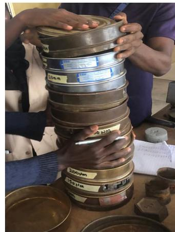
**Plate 1.** Set of Sieve Sizes Arranged in Descending Order
