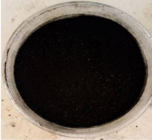
**Figure 3.** Balanite endocarp pod ash
