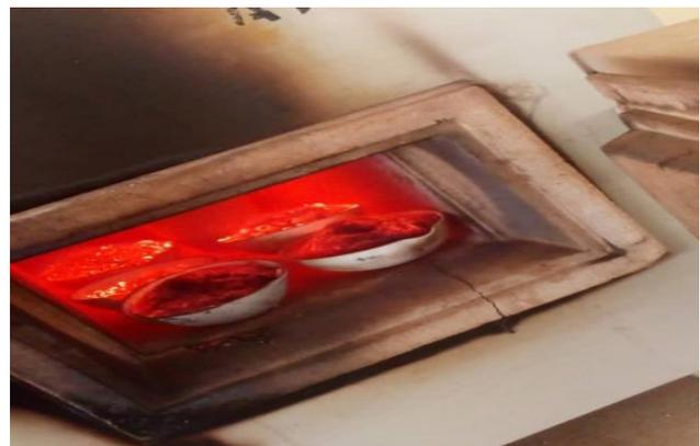
**Figure 2.** Calcination of balanite pod
