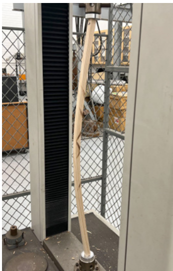
Figure 5. Specimen #6 buckling under compression.
