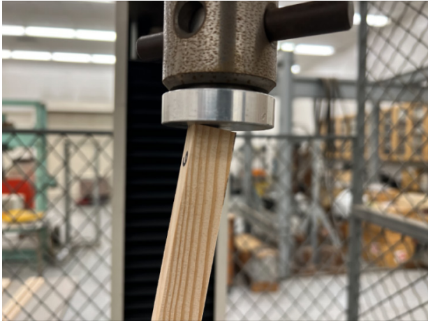
Figure 8. Upper crosshead support under loading.
