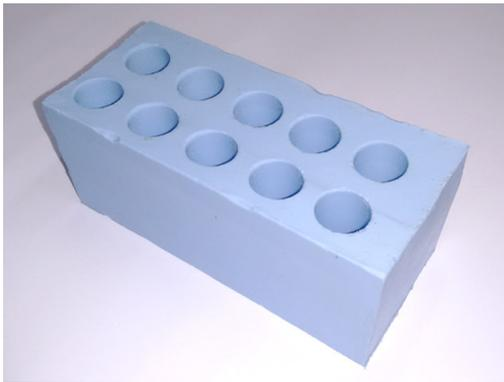
**Figure 5.** Silicon Mould Used to Manufacture Sample
