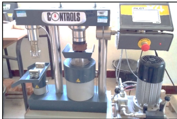
Figure 4. Compressive strength analysis of unfired clay-biopolymer bricks.
