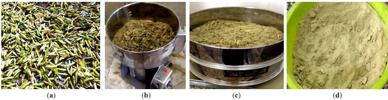
Figure 2. Biopolymer powder preparation from pea shell waste: (a) Collection and sun-drying; (b) Grinding; (c) Sieving; and (d) final powdered product.
