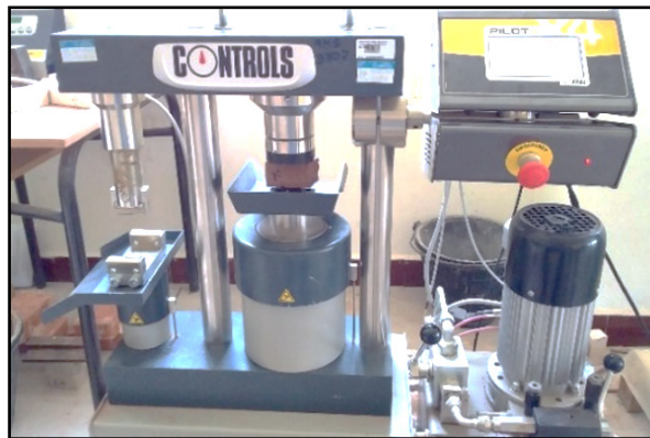
Figure 4. Compressive strength analysis of unfired clay-biopolymer bricks.
