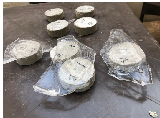
Figure 2. Frozen surfaces of the oiled mortars and dry surfaces of non-oiled mortars after every natural freezing cycle.
