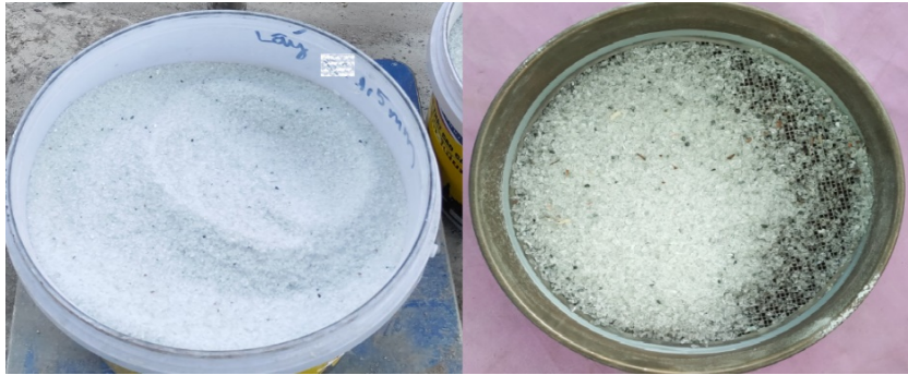
Figure 2. Recycled glass has been created: (a) Glass is filtered using various kinds of sieves; and (b) sieved glass aggregate.
