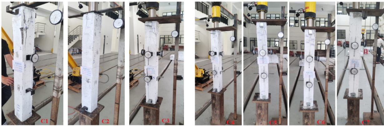
Figure 7. After tests, the shape of the column samples.
