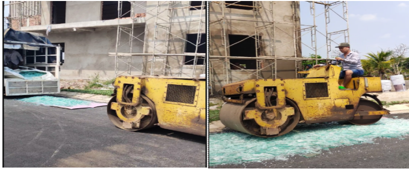
Figure 1. Glass is crushed into modules of sand aggregate.
