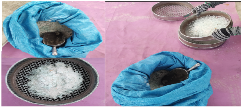
Figure 1. Glass is crushed into modules of sand aggregate.
