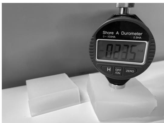
**Figure 3.** Hardness Shore A durometer.
