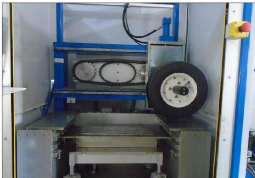
Figure 5. Compaction equipment according to EN 12697-33.
