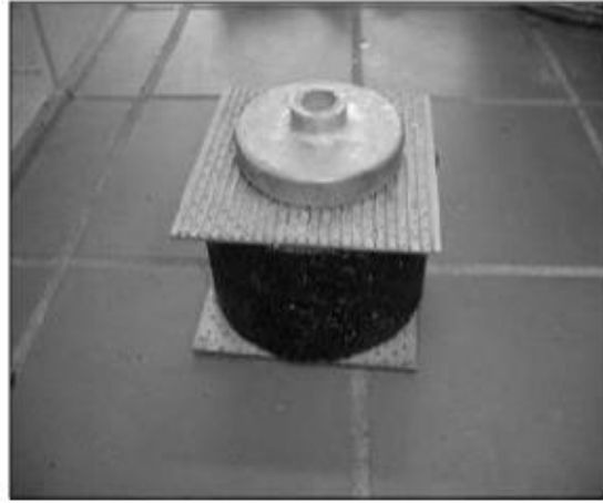
Figure 4. Position of the specimen between two metal plates, topped with a centrally recessed disc.
