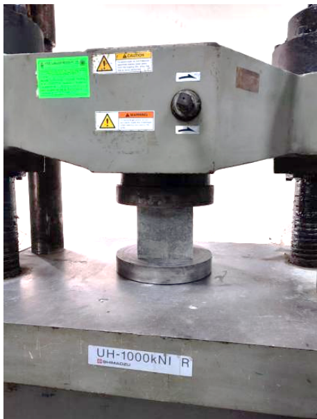
Figure 3. Universal Testing Machine (UTM-100T, SHIMADZU).
