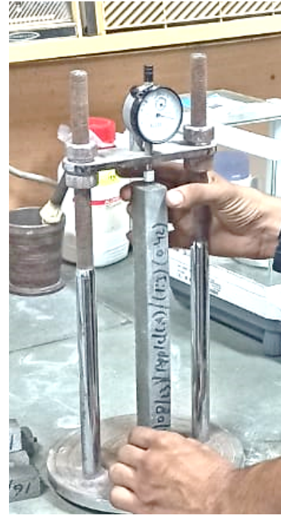
Figure 9. Drying shrinkage test apparatus.
