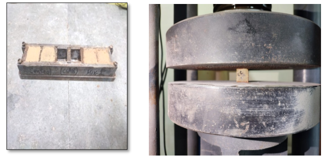
Figure 6. Casting and compressive strength testing of cube at 28 days.
