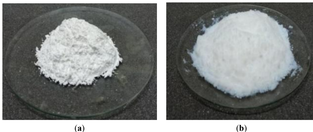
Figure 2. Raw materials (a) Pure Limestone, and (b) Fumed silica.
