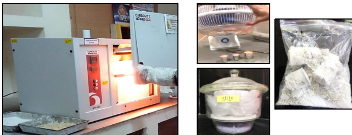
Figure 4. Operation of furnace during synthesis of alite, quenching in air, storage in desiccator of Silica Gel, and Alite sample.
