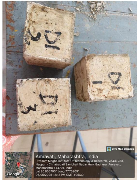
Figure 4. Concrete Samples Ready for Curing.
