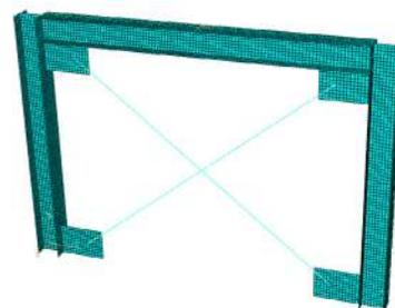
Figure 2. Finite Element Model of Moment Frame with Cable Brace
