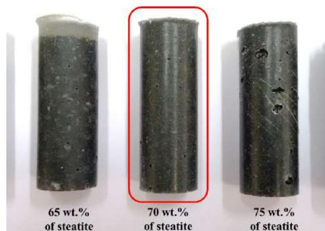
**Figure 8.** Polymer-based Composites with 65 wt.%, 70 wt.% and 75 wt.% of Steatite Inclusions
