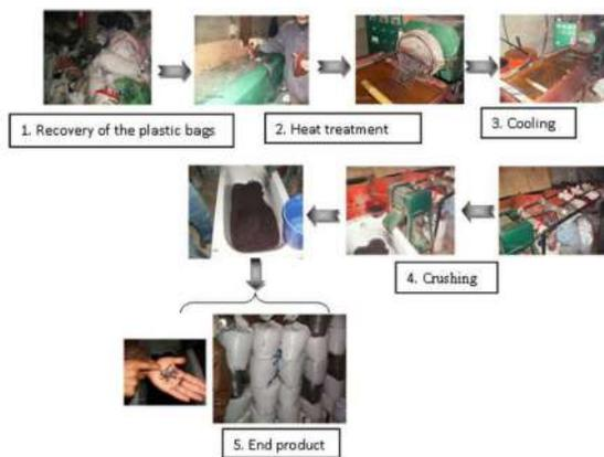
**Figure 2.2** Production of Aggregate from Plastic Waste
