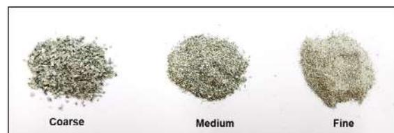
Figure 2. Steatite Classified in Coarse, Medium and Fine Monodispersed Particles.
