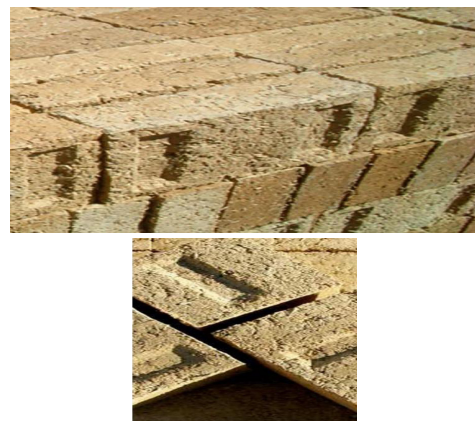
Figure 2. Brick made from Hempcrete [16]
