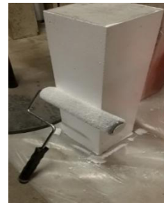
Figure 2. Application of liquid polymer coating to rectangular prism concrete sample.
