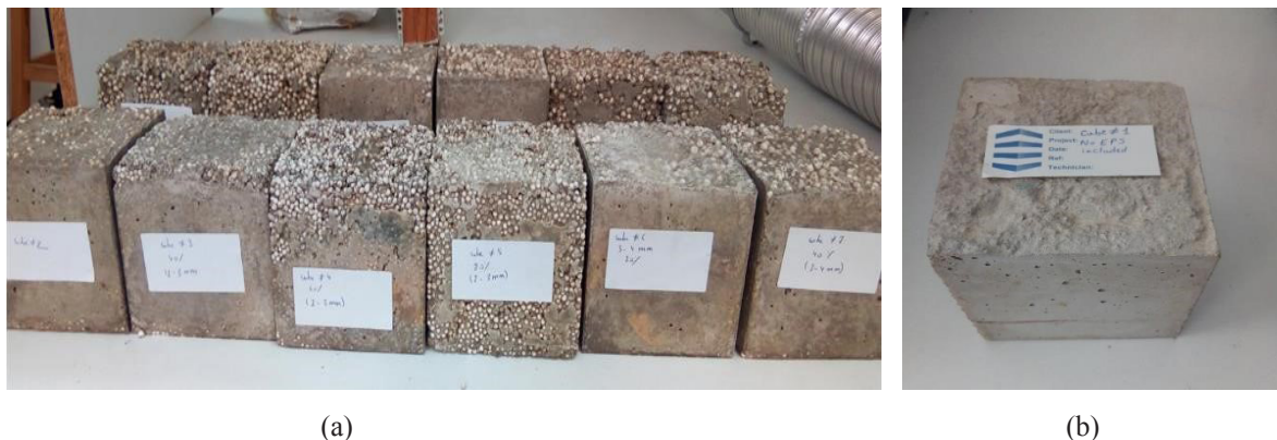
Figure 5. Cube 1 without EPS (a) and cubes 2-13 with different percentages and different diameters of EPS beads.
