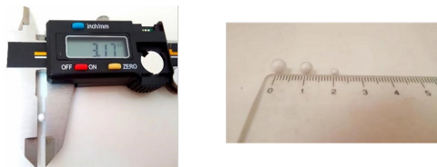
Figure 1. Three different dimensions of EPS aggregates.
