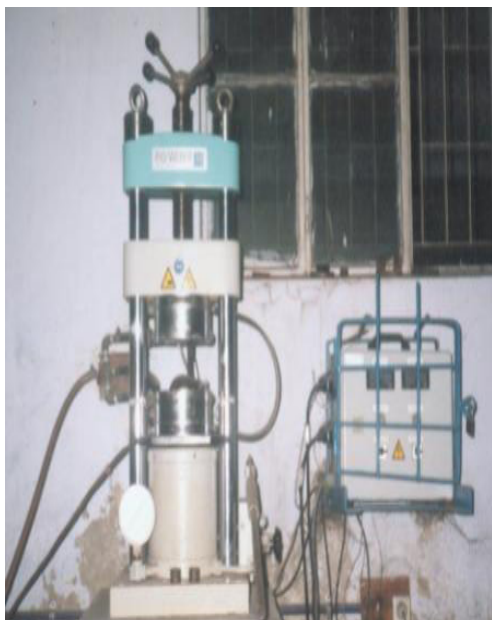
Figure 1. Weber Pressen hydraulic press.
