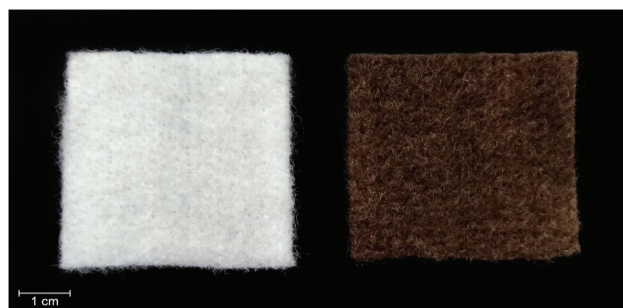
Figure 1. Geotextile Immersed in Sulphuric Acid 0.1 mol.L -1 Before (Left) and After Thermo-oxidation (Right).
