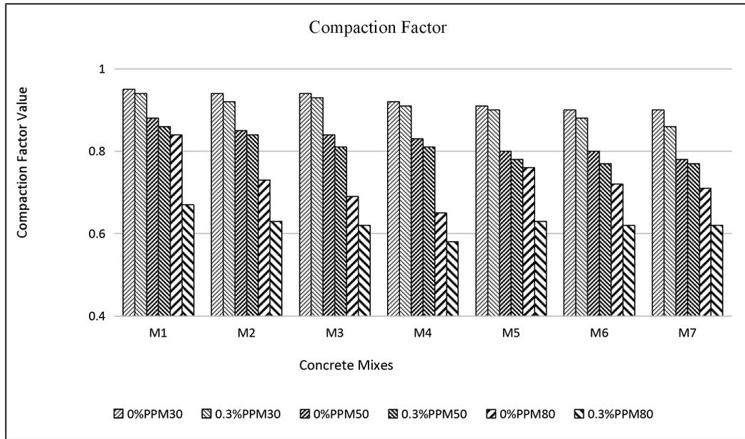
Figure 3. Compaction Factor Test results
