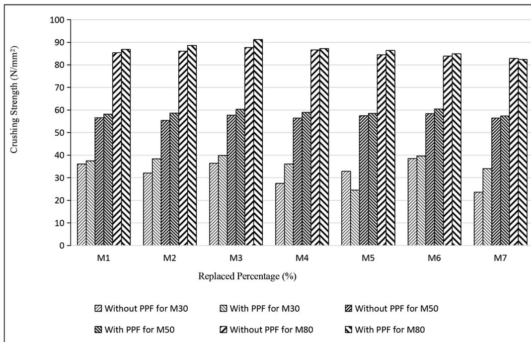
Figure 5. Graph showing Crushing strength of FS & CCW for 14 days curing
