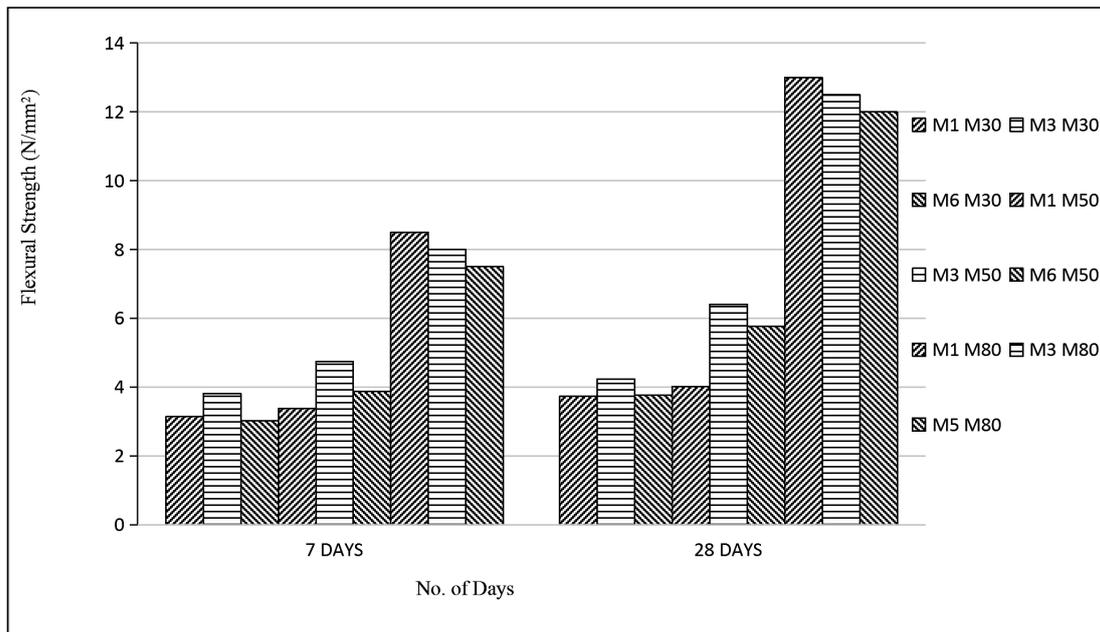
Figure 8. Graph showing Flexural strength of FS & CCW for 7 and 28 days curing
