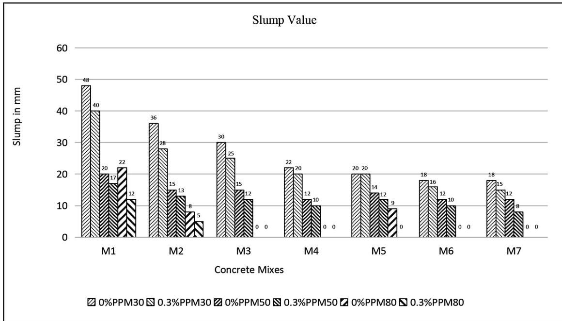
Figure 2. Graphical representation of slump test results
