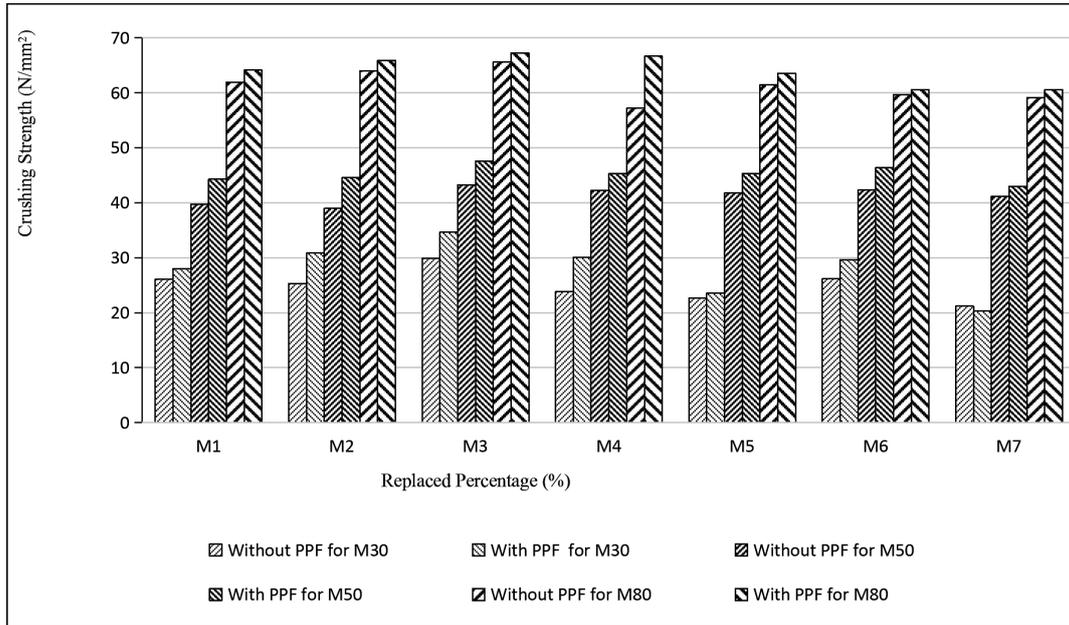
Figure 4. Graph showing Crushing strength of FS & CCW for 7 days curing
