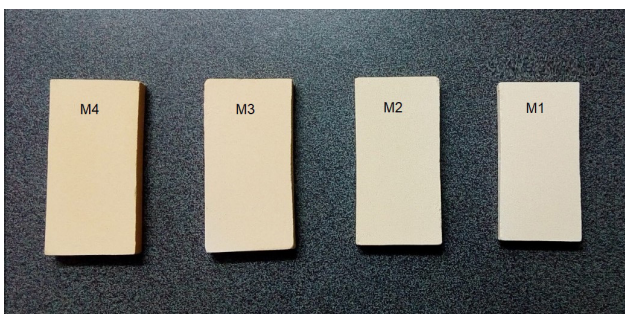
Figure 11. Aspect of samples fired at 1400 °C
