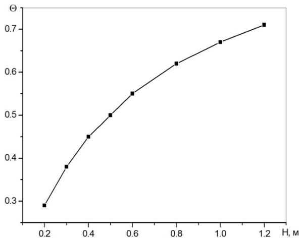
**Figure 5.** Temperature efficiency versus filling height
