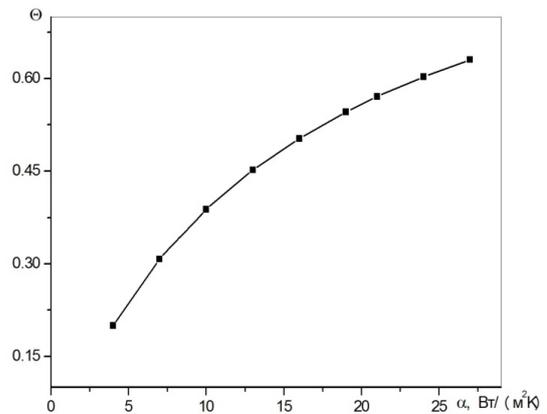
**Figure 7.** Temperature efficiency versus heat transfer coefficient
