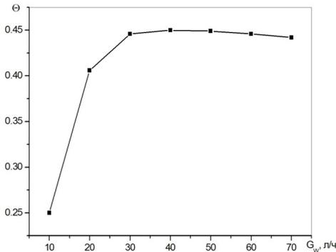
Figure 8. Temperature efficiency versus water flow rate
