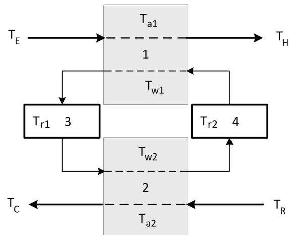
Figure 3. Flowchart of a regenerator with intermediate
