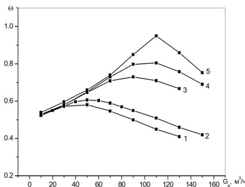
Figure 9. Temperature efficiency versus air flow rate for filling height: 1 - H=0.4 m, 2 - 0.5 m, 3 - 1.2 m, 4 - 2 m; 5 -
