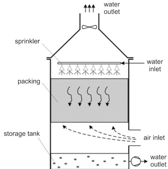
**Figure 2.** Counterflow packed column
