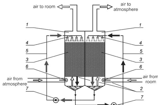
**Figure 1.** Scheme of air heat regenerator with intermediate heat carrier: 1 - column body, 2 - grate, 3 - packing, 4 - sprinkler, 5 - pipeline, 6 - air ventilator, 7 - water pump.
