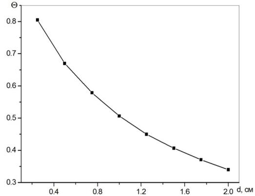
**Figure 6.** Temperature efficiency versus packing diameter
