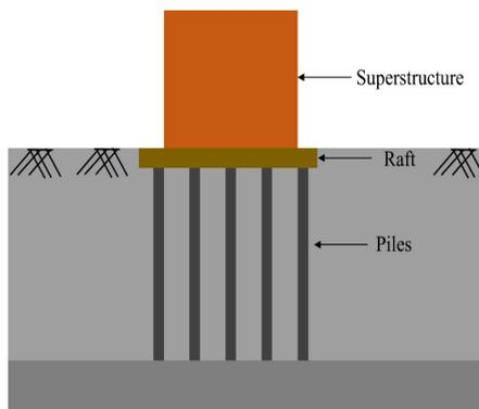
Figure 2. Piled raft foundation
