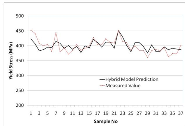
Figure 3. Validation of YS for Micro-alloyed Steel
