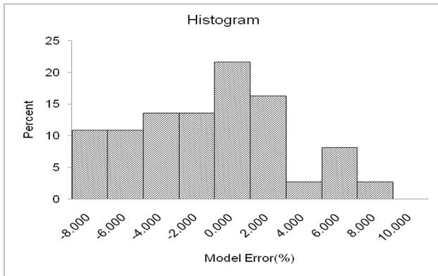
**Figure 4.** Histogram Showing YS Model Error (%) for Micro-alloyed Steel
