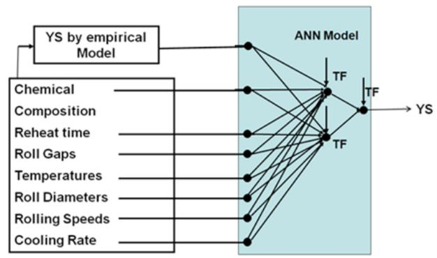
Figure 1. Conceptual Diagram of Hybrid Model
