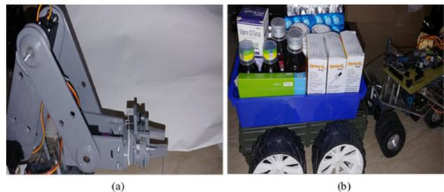
**Figure 11.** Robotic arm and UGV (a) Robotic arm with 5 degrees of freedom <sup>[6]</sup> used for assistance in critical circumstances (b) Unmanned vehicle carrying drugs for contactless delivery.
