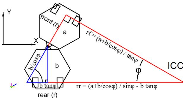
**Figure7.** Rotational radius of a vehicle with articulated steering of angle  $\phi$ , front length as  $a$ , and rear length as  $b$ .
