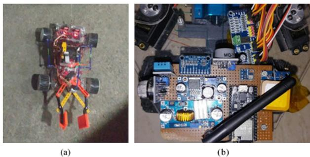
**Figure 9.** UGV (a) First prototype of the mechanical system for UGV. (b) Its main control boards.
