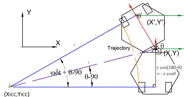
**Figure 8.** Rotation of vehicle around ICC with angle  $\omega\delta t$ . Here position changes from  $(x, y, \theta)$  to  $(x', y', \theta')$  which is represented in a global coordinate system (top left). The ICC coordinates are  $(x - r \sin\theta, y + r \cos\theta)$ .
