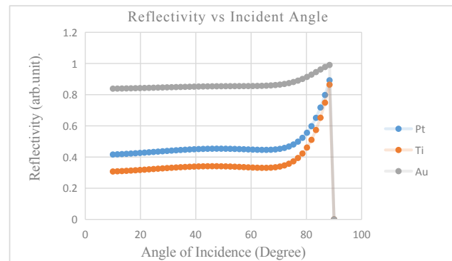
Figure 9. Comparison of Reflectivity for Au, Pt and Ti Metal
