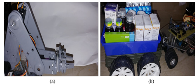
Figure 11. Robotic arm and UGV (a) Robotic arm with 5 degrees of freedom [6] used for assistance in critical circumstances (b) Unmanned vehicle carrying drugs for contactless delivery.
