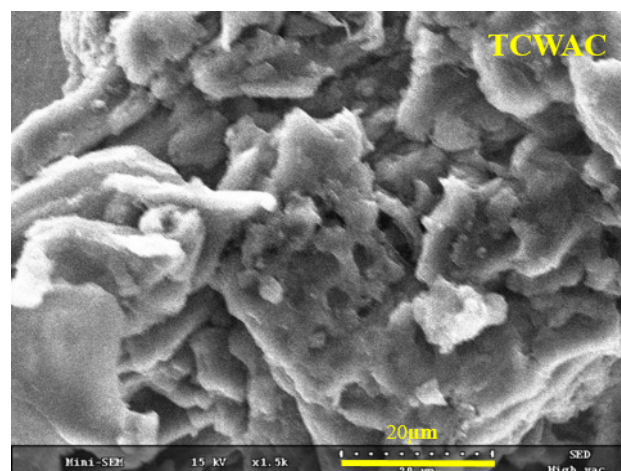
Figure 2. SEM Image of TCWAC Showing Irregular, Interconnected Pores with a Rough Surface (Scale Bar = 20 \mu\text{m} ).
