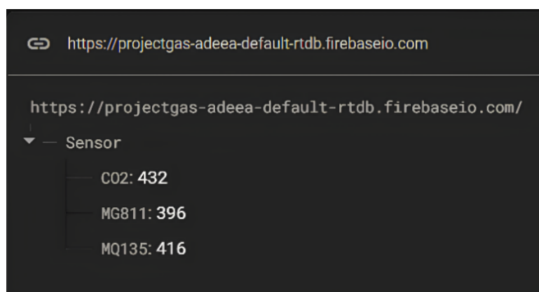
Figure 4. Real-Time CO 2 Data Display on Firebase Realtime Database at Jl. AP. Pettarani, 20 Meters Height, 16:00.
