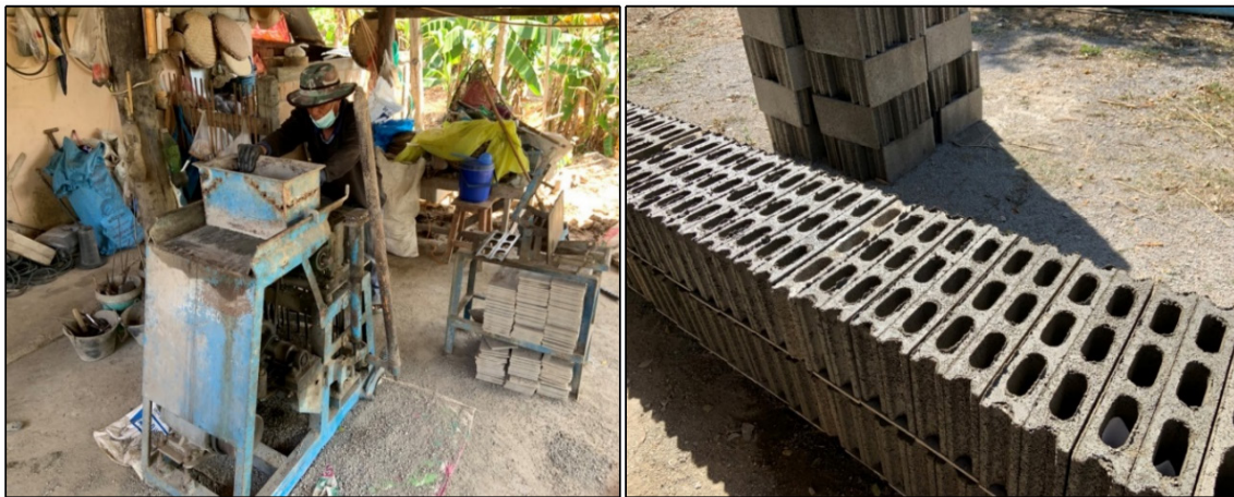
Figure 5. Development of waste ash for producing concrete blocks.
