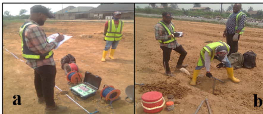
Figure 3. (a) ERT survey investigation; (b) auger borehole soil sampling.
