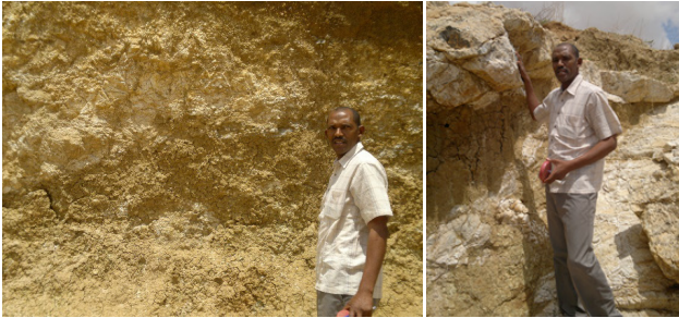
Figure 4. Weathering and fractured profile on gneiss of the study area (Abu Zabad - Torda)
