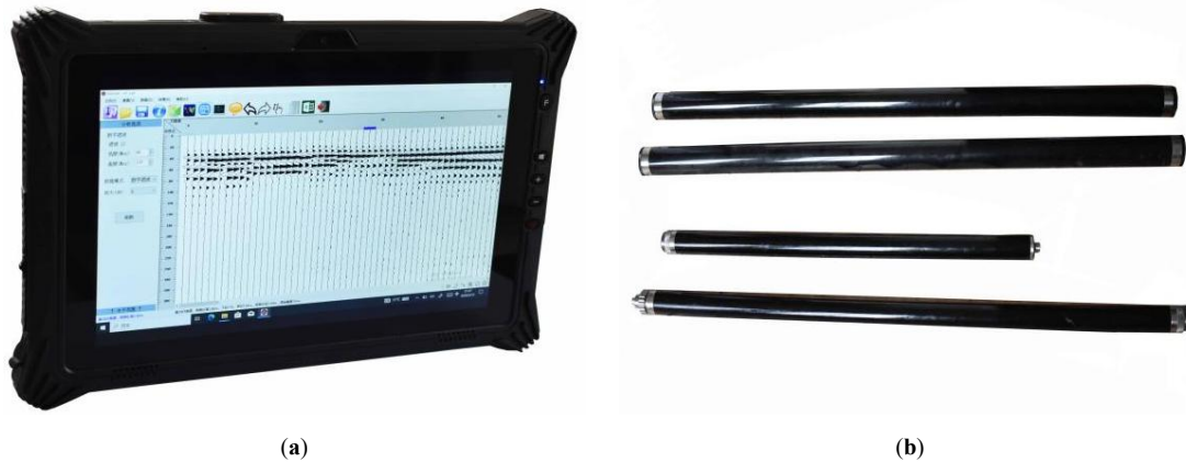
Figure 1. Single-hole impulse borehole radar system: (a) acquisition and control computer; (b) borehole radar probe.
