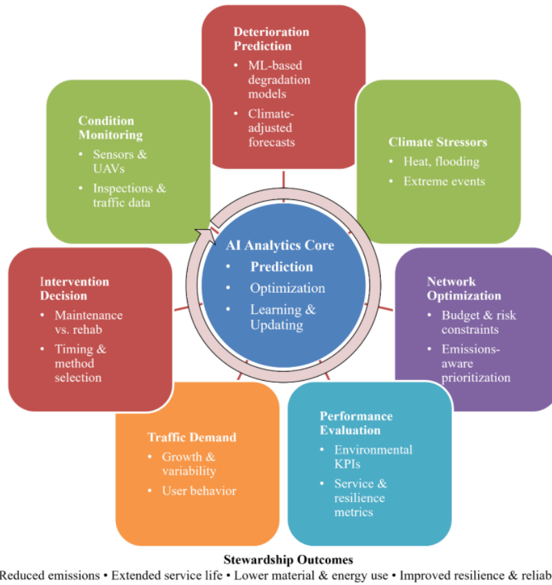
Figure 3. Closed-loop, AI-supported adaptive asset management for long-term environmental stewardship, integrating monitoring, deterioration prediction, network optimization, intervention selection, and performance evaluation under traffic and climate uncertainty.
