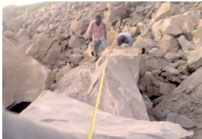
Figure 5. The photograph of the block size measurement using the line method.
