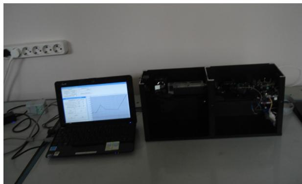
**Figure 1.** A combined Led spectrophotometer and spectroellipsometer.
