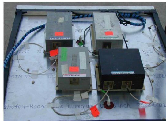
Figure 2. Several samples of microwave radiometers with a wavelength of 2.25, 6, 18/21 and 30 cm, were produced by a special design office of the Kotelnikov Institute of Radioengineering and Electronics RAS [10–12].
