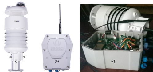
Figure 4. IoT device: (a) weather station, (b) sensor hub 4G data Logger, (c) device in setup and configuration process.
