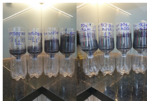
Figure 4. Adsorption filter for pig feed water and inorganic fertilizer.
