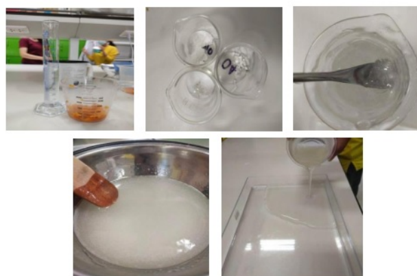
Figure 2. Procedure for the Preparation of Biodegradable Films (1. Add 140 mL of distilled water 2. Prepare xylitol, calcium chloride, and alginate 3. Dissolve 1.2, 1.8, and 2.4 grams of alginate, respectively 4. Stir manually 5. Pour into the mold) [9] .
