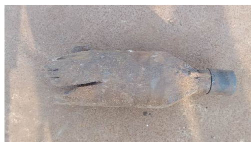
Figure 11. Artisanal drill bit.
