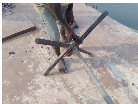
Figure 18. Assembly of the bit and the drill rod.
