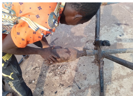
Figure 19. Assembly of the flexible tube and the L-shaped tube.
