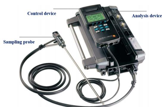
**Figure 4.** Testo 350 XL device for NO<sub>x</sub> emission analysis.
