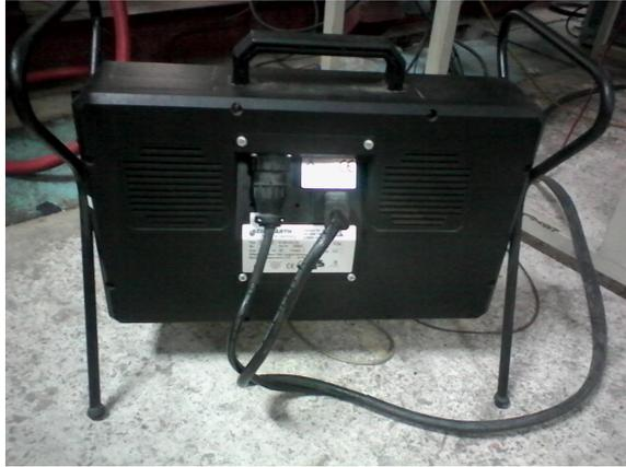
Figure 5. Msa-pc-se. nr 00601 Smoke Opacity Meter.
