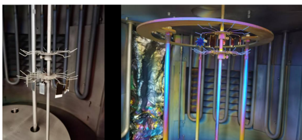
Figure 6. Color difference of the suspension bracket before and after magnetron sputtering in the furnace cavity.
