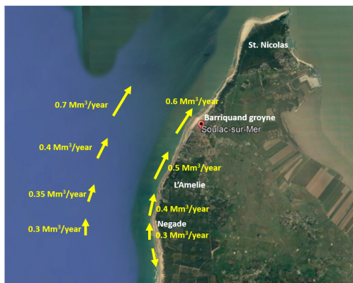
Figure 10. Net annual longshore sand transport values in shoreface zone (seaward of -5 \text{ m} depth) and in surf zone (landward of -5 \text{ m} depth line).
