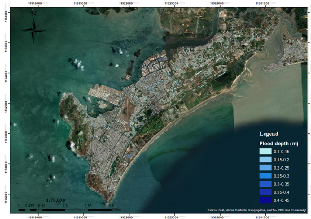
Figure 7. Simulation Results of Urban Flooding Based on the Representative Rainfall Event of June 19, 2020 with Color Bar Indicates Flood Depth (m).
