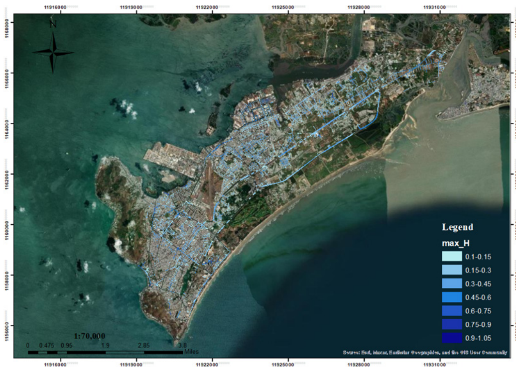
Figure 10. Simulated Urban Flooding Extent and Depth (m) for a 10-Year Return Period Rainfall Event. Color Bar Indicates Water Depth Ranges.
