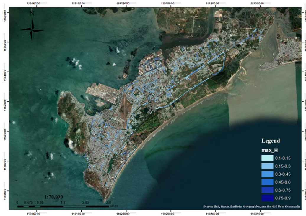
Figure 9. Simulated Urban Flooding Extent and Depth (m) for a 5-Year Return Period Rainfall Event with Color Bar Indicates Water Depth Ranges.
