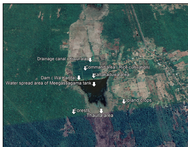
Figure 2. Part of Thirappane tank cascade showing Meegassagama tank and its prominent components (Google Earth map taken during dry season)
